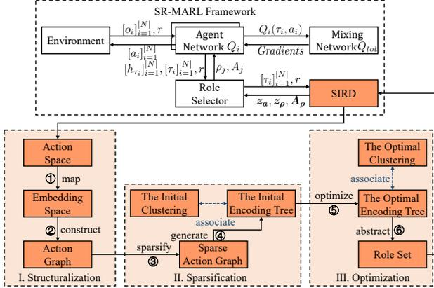
Figure 1: The overall framework of the SR-MARL.
